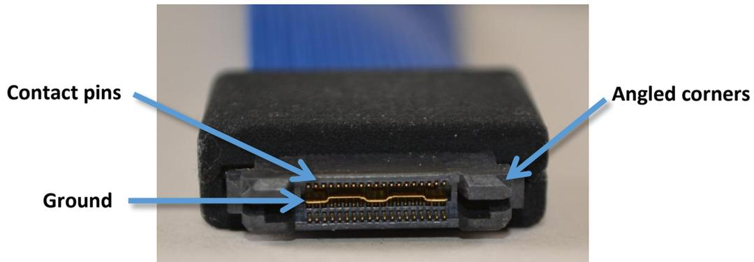
2. Note the shape inside the Mictor socket. The Mictor probe can only be inserted one way...
