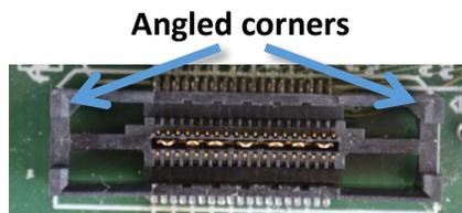
3. Gently press the probe straight down into the Mictor socket until it's fully seated....
