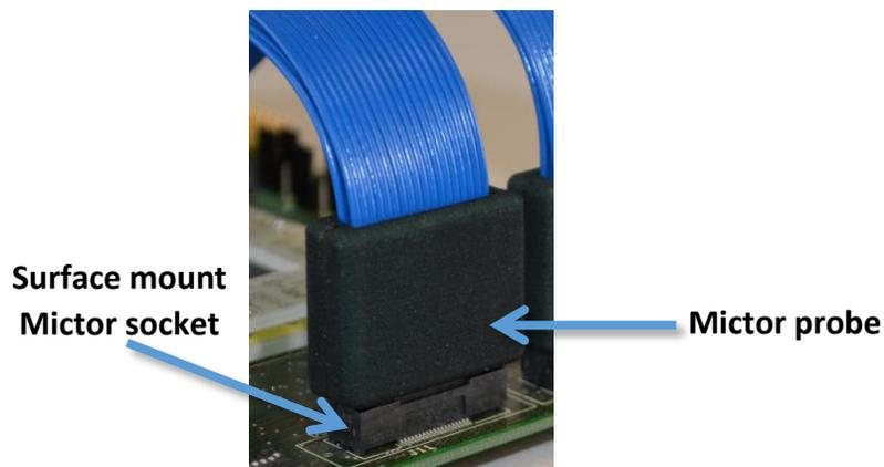
4. Whenever possible, the blue ribbon cable should remain straight and motionless as possible. Motion, twists, and excessive flexing can apply torque and pressure on the probe and compromise the pin connections.
